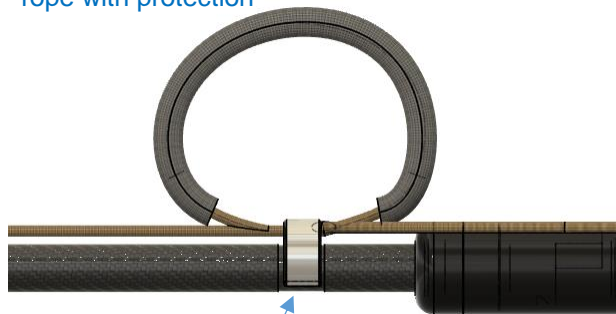
Lower Rope Clip (should be placed in dedicated groove in guide tube)
